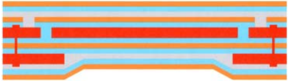
Double Layer Flex With Two Conductive Ink Planes
