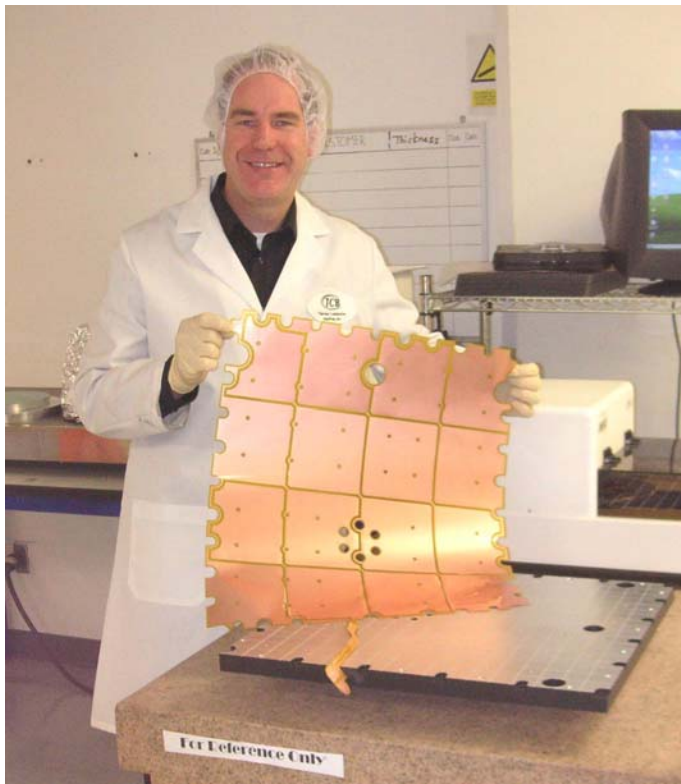
Figure 4 Wayne Simpson, President of TCB, with the reverse engineered flex circuit.
